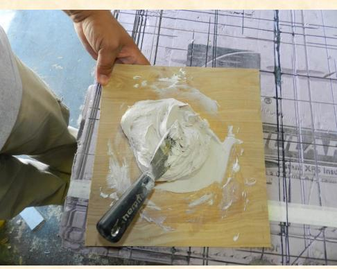
Next, we suggest using pro series transparent knife grade polyester with coloring paste to join your mitered edges together. Matching the dye to your stone can be difficult. We suggest you test your coloring before applying.
