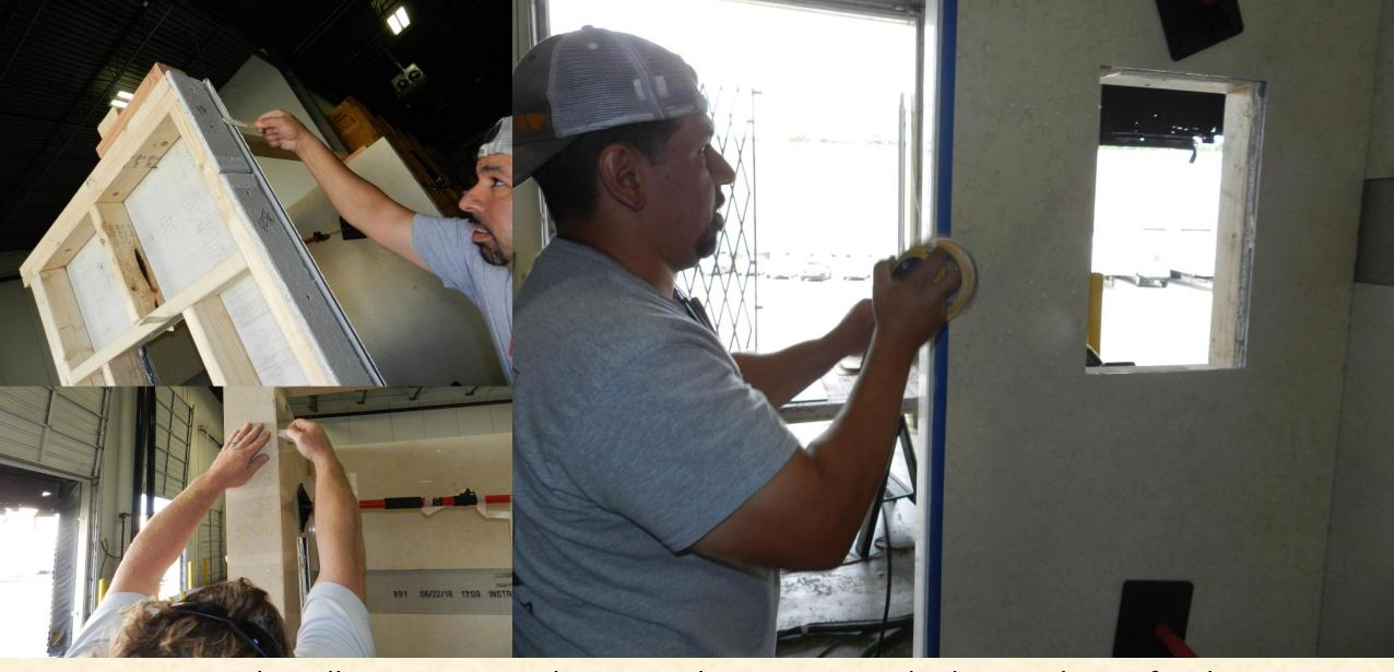
Smear the adhesive paste in between the two mitered edges and tape firmly together. Once dried, you gently sand away the excess with a series of very high grit sandpaper.
